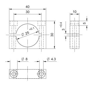
2 Allen head screws M4 x 35 mm (DIN 912, A2) and 2 spring rings (DIN 127, A2) are included in the scope of delivery of the MB25.
