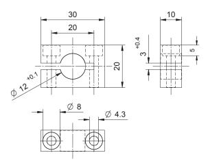
2 Allen head screws M4x25 mm are included in the scope of delivery.
