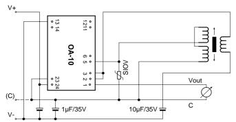
Connection (C) is not required for an unsymmetrical supply voltage.
