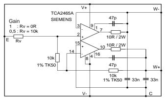
Connection (C) is not required for an unsymmetrical supply voltage.
