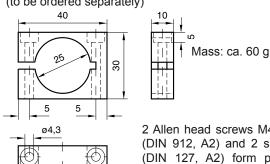
2 Allen head screws M4 x 35 mm (DIN 912, A2) and 2 spring rings (DIN 127, A2) form part of the MB25's scope of delivery.
