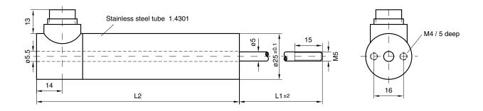
Version with ball joint on plunger (KV) (without rod guide)
