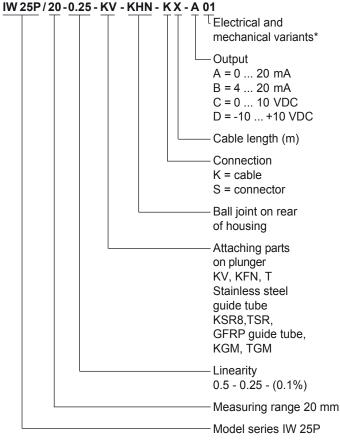
The basic versions according to the data sheet have the number 01. Deviations are identified with a variant number and are documented in the factory.
