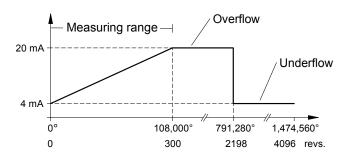
Note: If the measuring range cannot be found directly due to sensor shaft rotation (as the sensor system is in the overflow or underflow range), the rotary encoder can be pre-set with the aid of the MFPs. As a result, the rotary encoder jumps to the centre of the measuring range.
