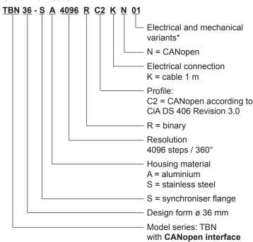
\* The basic versions according to the data sheet bear the number 01. Deviations are identified with a variant number and are documented in the factory.
